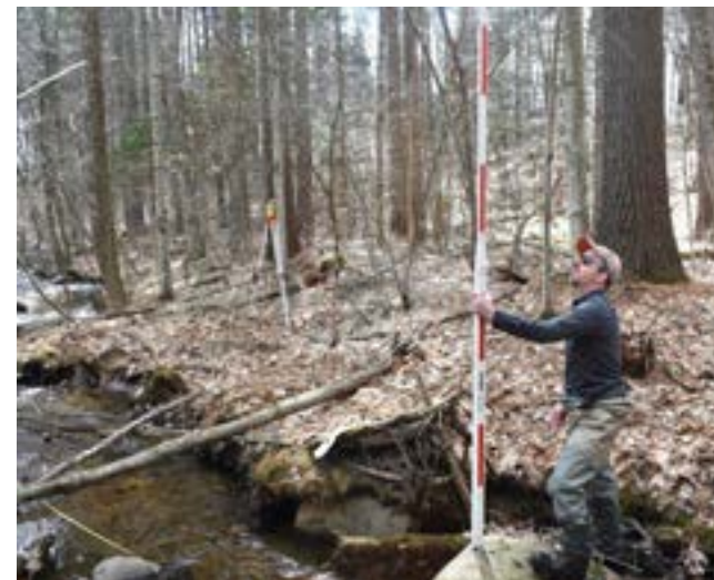
Stream Restoration Manager, Gary Henry, measuring a temporary benchmark as part of a geomorphic survey of a tributary to the West Branch Ausable River
