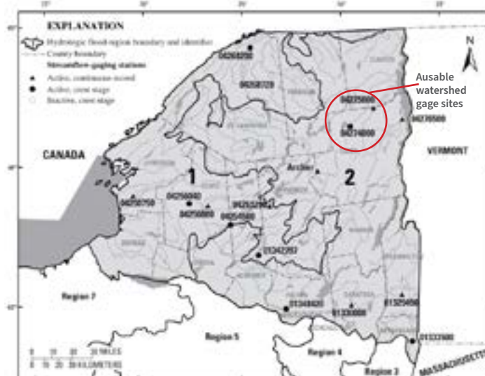
Map of the area used to develop regional bankfull discharge and hydraulic geometry relationships in Northern New York (from Mulvihill et al., 2007). Gage sites in the Ausable watershed are circled in red.
