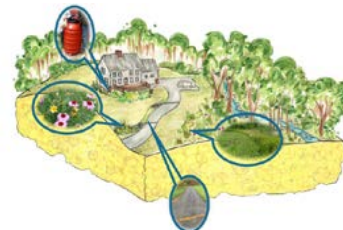
Diagram showing stormwater implementation projects (rain barrel, rain garden, waterbar, no-mow and low-mow zones) identified through a theoretical Storm Smart assessment on private residential land.
