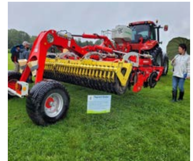
Tegosem seeder and roller assembly on Pottinger Terradisc— August 16th Field Meeting
