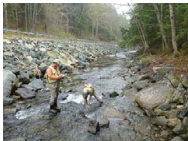
Pebble count for Phase 2 assessment on the Green River in Halifax, VT
