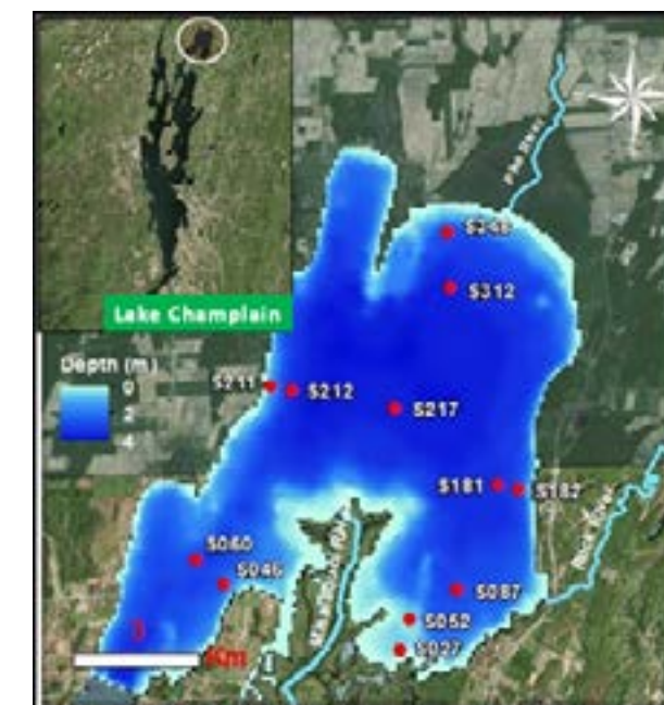
Figure 1. MB site and bathymetry map with sample core locations (red dots) where sectioned cores (to 10 cm) have been analyzed for P inventories at 4 time points in 2013 (June–Sept.). At point S087, there are biweekly time series of sediment P inventories in 2013-14 and 2014-2015. All points have coincident water column physical, chemical and biological data (Table 1).
